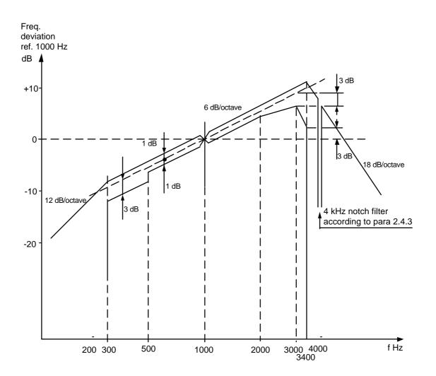
Fig. 2.2 Audio frequency response of transmitter
