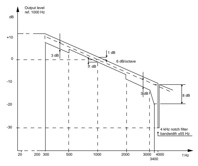
Fig. 2.4 Receiver audio output level as a function of modulation frequency at constant frequency deviation
