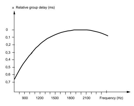
Fig. 6.2 Group delay of distortion circuit
