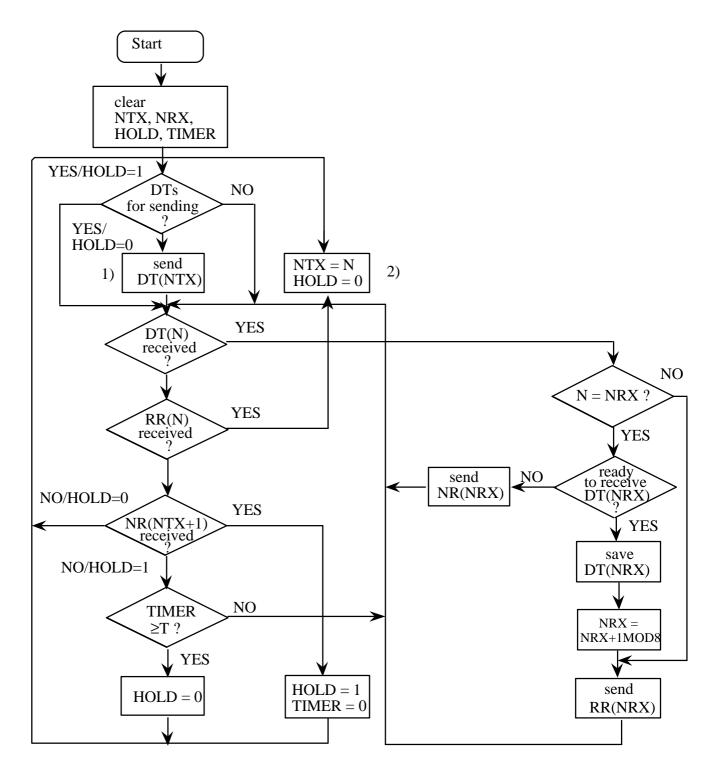
1) DT(NTX) to DT(NTX+3) are put to repeated transmission. Transmission of frames continues in numerical order.
