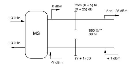
Figure 5. Measuring levels for connecting a 4-wire equipment to a mobile station
