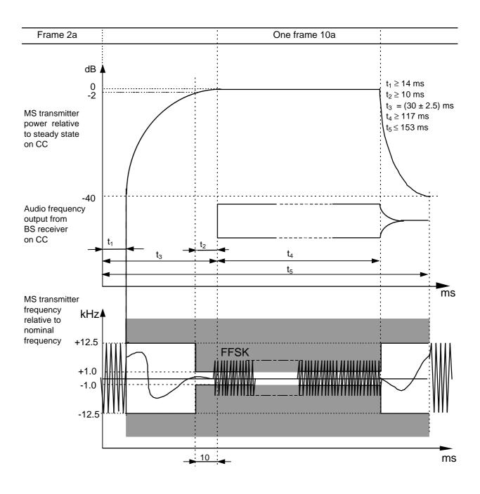
Fig. 6.3 Transmitter frequency transient behaviour, start up and decay times
