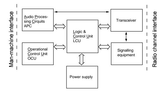
Fig. 5.1 Logic connections between the LCU and other entities in the MS
