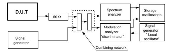
Fig. 6.4 Measurement arrangement
