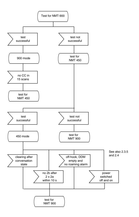
*Figure 2. State diagram for switching between NMT-900 and NMT-450 (See definitions in paragraph 2.1)*
