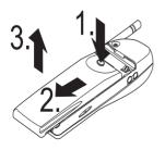
(3) Release the SIM card holder by sliding the catch in the OPEN direction.
